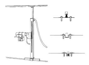
Figure 3: Tube support for design B.
