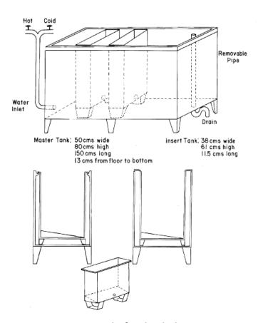
Figure 9: Tanks for the darkroom
