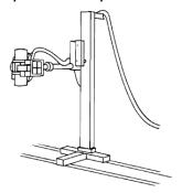
Figure 4: A floor rail mounted tube.
