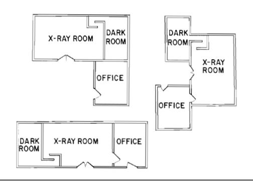
Figure 1: Alternative room layouts for a radiographic suite
